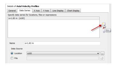
Add a third data series by clicking on the "New" icon and repeating the steps for x=6.045 m. You should then have three items in the Data Series tab.
