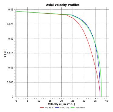
We notice that the flow accelerates due to the heating. As air is heated, its density decreases. So the velocity has to increase to maintain the same mass flow rate.
