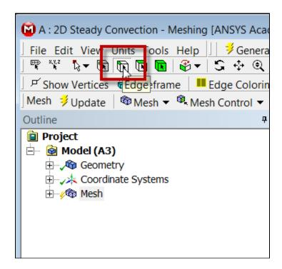
Select **Zoom to Fit** as shown in the snapshot below to fit the entire geometry in the graphics window. Hold down the left mouse button and drag over the four horizontal edges (two top and two bottom). The surfaces will be highlighted in green when they've been selected.
