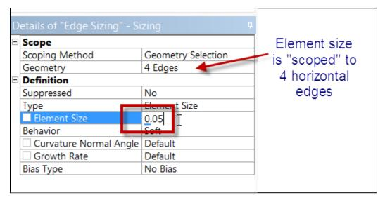
Now, we will create an edge sizing for the vertical edges of the geometry. Create another edge sizing, and this time, choose the left and right vertical edges of the geometry by holding down the *Ctrl* key and selecting each of them, and go to *Geometry > Apply*. Change the *Type* to *Number of Divisions*. Next, specify *Number of Divisions* to 30. Note that one can specify the Element Size or Number of Divisions depending on which is more convenient.
